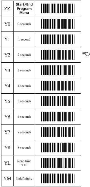
**Read Time Settings** - the length of the period that the reader is ON after the trigger switch is pressed, or (in multiple or continuous read mode) after a label has been read. Selecting a read time of 0 means that the reader will stay ON as long as the trigger switch is being pressed. Selecting a read time for readers without a trigger switch, or when the trigger switch is disabled, has no effect.
