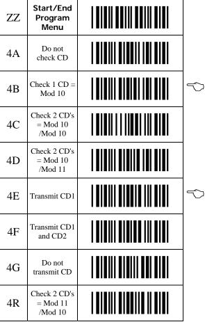
**MSI Plessey** is a variable length symbology with one or two optional check digit calculations CD1 and CD2 and non printable start/stop characters. Supported characters include numeric digits 0 through 9.
